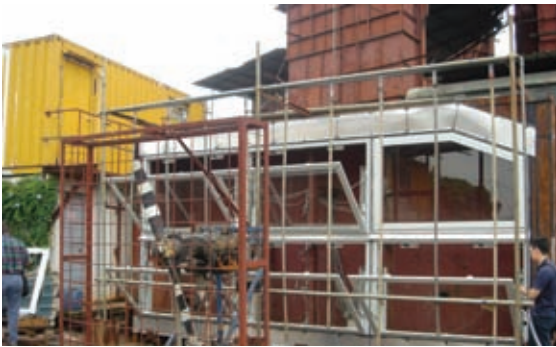
Rain test rig for the ventilators to be installed at Sky Plaza, Hong Kong
