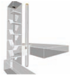
Colt Shaft | ACTIVE FAN SMOKE EXTRACTION SYSTEM to reduce space requirements and increase extraction capacity – for shafts
