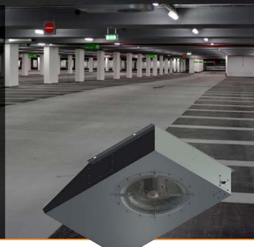
Colt Cyclone is a low profile, high velocity induction jet fan intended to control air movement and direct polluted air and smoke towards the extract positions in a car park or underground service area.
